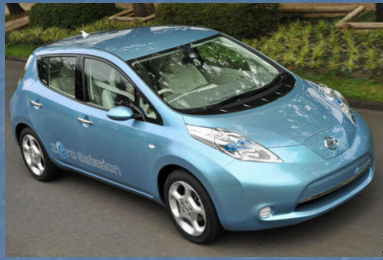
Nissan Leaf Five passenger Base Price: $25,280 Range: ~100 miles Performance: 0-60 ~ 9 sec., 90 mph max
