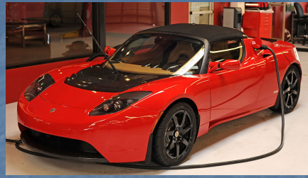
Tesla Roadster Two seater sports car Base Price: $101,500 Range: ~244 miles Performance: 0-60 ~ 3.7 sec., 125 mph (electronic governor)
