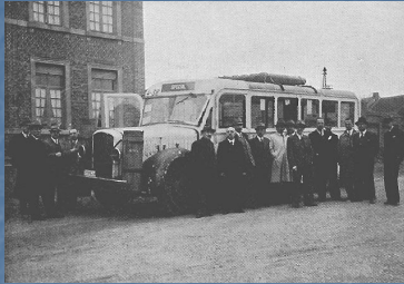
Anhydrous-ammonia-powered bus used in Belgium during WWII
